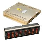
The 506 series provides up to 32 channels of airframe system condition. The LED backlit display head is a low-profile design, with the control assembly ("brain box") mounted remotely for ease of installation in cockpits with depth limits on the instrument panel. The control assembly provides input conditioning and master caution/master warning (MCMW) logic, and indication control. The control assembly is capable of driving two 506 display heads in parallel.
