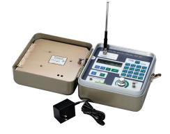
AvtechTyee's CTS-700 Ramp Tester contains a built in transmitter and uses VHF or HF signals, transmitted directly to the aircraft, to conveniently test the aircrafts SELCAL system
