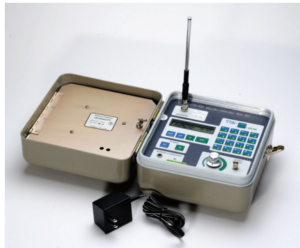
AvtechTyee's battery powered CTS-700 Ramp Tester contains a built in transmitter and uses VHF or HF signals, transmitted directly to the aircraft, to conveniently test the SELCAL system at the aircraft without any intervention from the tower or ARINC
