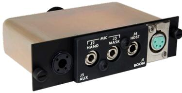
Avtech's 5127 series of jack panel feature both high and low impedance microphone inputs, a built in high gain military style dynamic microphone amplifier and an output transformer to switch between high and low impedance headsets. Jacking provisions are provided for various types of microphone styles. The 5127 is certified and issued as standard equipment aboard the CASA and IPTN CN-235 aircraft, both commercial and military versions.
