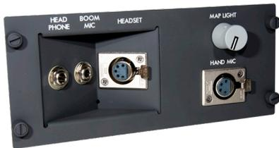
Avtech's 5775 series jack panel is the 1st Officer's jack panel used on Boeing's 787 aircraft. The panel features hand mic jacks and plugs which prevent the user from plugging in two sets of jacks by positioning the jack in a manner where it is impossible to plug both in simultaneously. This technique prevents the loading effects of plugging in multiple headsets into one input or output. The panel also features the inclusion of a map light adjustment.
