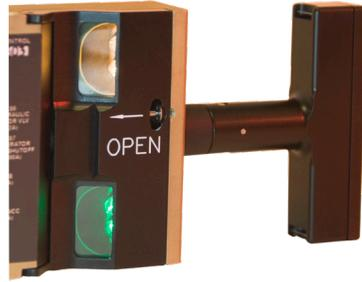
The 380 series fire switch is utilized on the C-17 Military cargo aircraft. The 380 features an integrated NVIS green and standard white panel floodlight. The handle is pulled out to "ARM" and rotated left or right to discharge the fire bottles.
