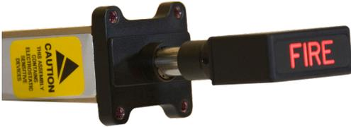
The 44607 fire switch is designed for the BA-609 aircraft. The 44607 features a pull to arm mechanism, and a fire bottle discharge by rotating the handle 30 degrees to the left or right.
