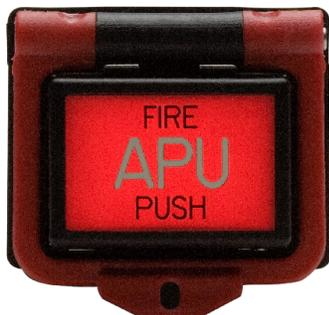
The 481 series is an 8-pole alternate action switch assembly designed for the Dornier 328 aircraft. The switch guard locks the button from being pushed until it is lifted up to a detent position. The switch is activated by pushing the button in .10". Once released, the button activates the electro-mechanical switch to activate the circuit. The 481 switch has been utilized for APU fire bottle and Cargo area fire suppression systems.
