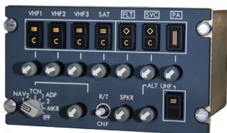
Another successful modification of Avtech's standard 737NG system is the 5347 P8 Poseidon system. This system required a reduced panel Audio Control Panel, military radio interfaces, custom switch legends and a UHF interface.
