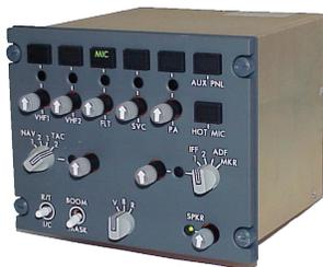
The 5346 panel is a modification of Avtech's successful 737NG system and was modified to provide the needed interfaces to military radios such as Tacan and IFF. The system also acts as a bridge from the secured communications of the mission control personnel to the unsecured communications in the flight deck.
