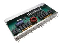
AvtechTyee offers the model TU202X12 as a replacement to Vibrasponders used in early model Motorola SELCAL decoders. Being mechanical devices, Vibrasponders are subject to wear and false triggering
