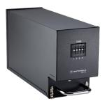
The N1401C (part number NA134D2) is a 2 channel, 16 tone SELCAL encoder packaged in a 1/2 ATR short case per ARINC specification 404A
