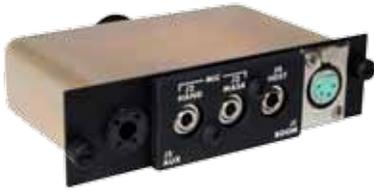
AvtechTyee's 5127 series of jack panel feature both high and low impedance microphone inputs, a built in high gain military style dynamic microphone amplifier and an output transformer to switch between high and low impedance headsets. Jacking provisions are provided for various types of microphone styles. The 5127 is certified and issued as standard equipment aboard the CASA and IPTN CN-235 aircraft, both commercial and military versions.
