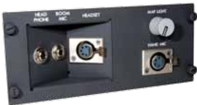
AvtechTyee's 5775 series jack panel is the 1st Officer's jack panel is supplied to Rockwell Collins and used on the Boeing 787 aircraft. The panel features hand mic jacks and plugs which prevent the user from plugging in two sets of jacks by positioning the jack in a manner where it is impossible to plug both in simultaneously. This technique prevents the loading effects of plugging in multiple headsets into one input or output. The panel also features the inclusion of a map light adjustment.
