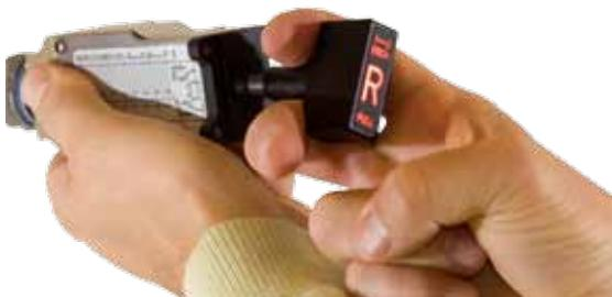
The 44640 fire switch is designed for the Raytheon Hawker Horizon aircraft. The 44640 comes in versions for left and right engine (L, R) and features a pull to arm mechanism, and the ability to fire two fire bottles by rotating left for #1, to right for #2 bottle.
