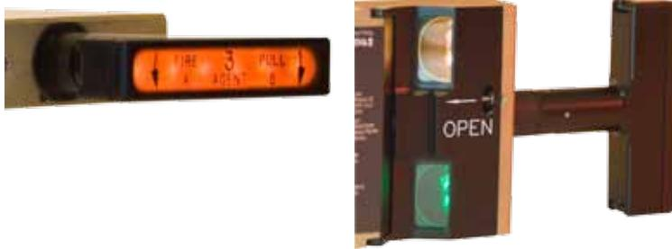
The 380 series fire switch is utilized on the C-17 Military cargo aircraft. The 380 features an integrated NVIS green and standard white panel floodlight. The handle is pulled out to "ARM" and rotated left or right to discharge the fire bottles.
