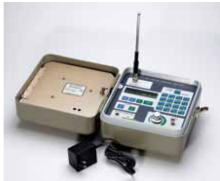
AvtechTye's battery powered CTS-700 Ramp Tester contains a built in transmitter and uses VHF or HF signals, transmitted directly to the aircraft, to conveniently test the SELCAL system at the aircraft without any intervention from the tower or ARINC
