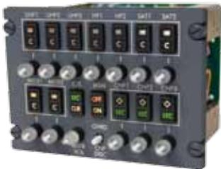
AvtechTye's 5348 panel acts as a control panel for the mission critical systems installed in the P8 Poseidon aircraft. It interfaces directly with secure voice systems
