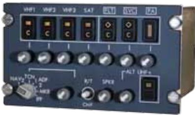
Another successful modification of AvtechTye's standard 737NG system is the 5347 P8 Poseidon system. This system required a reduced panel Audio Control Panel, military radio interfaces, custom switch legends and a UHF interface.
