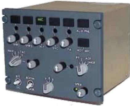
The 5346 panel is a modification of AvtechTye's successful 737NG system and was modified to provide the needed interfaces to military radios such as Tacan and IFF. The system also acts as a bridge from the secured communications of the mission control personnel to the unsecured communications in the flight deck.
